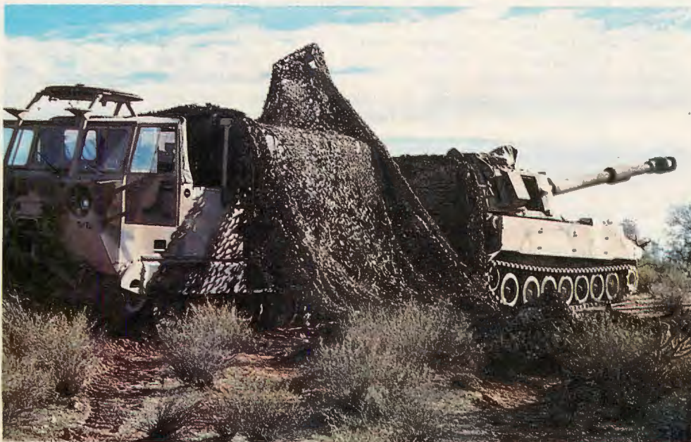
ABOVE: M109A3 155mm self-propelled howitzer is fitted with infrared night-vision equipment. Maximum range is 14,600 meters. BELOW: M109 of Arizona Army National Guard fires at Florence, Ariz., gunnery range.
